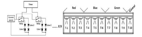
Fig. 1. LED Panel with 10 sections and Timer circuit for timing control
